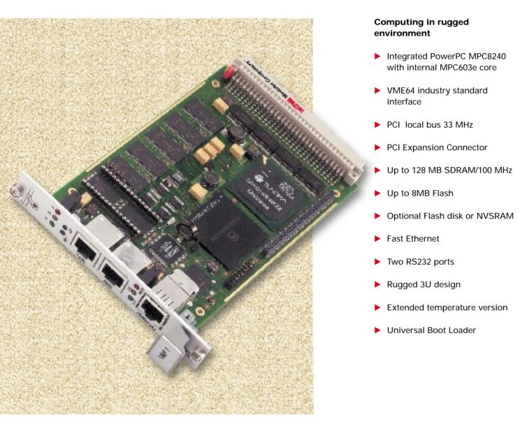
A well-balanced design achieving a maximum of computer performance versus power dissipation, realized using the highly integrated MPC8240 PowerPC, embedded in a rugged design.
